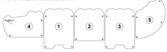
Drill the holes on the wall using an 8mm drill bit. Drill a hole 45mm in depth.
