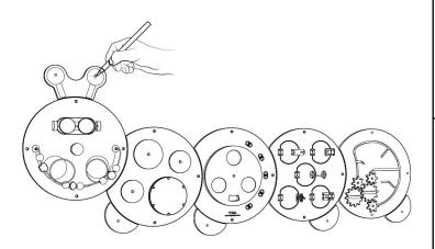
2 Drill the holes on the wall using an 8mm drill bit.Drill a hole 45mm in depth.
