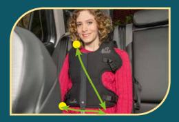
**3**-point harness ensures safety ALWAYS use together with the vehicle's own 3-point seat belt
