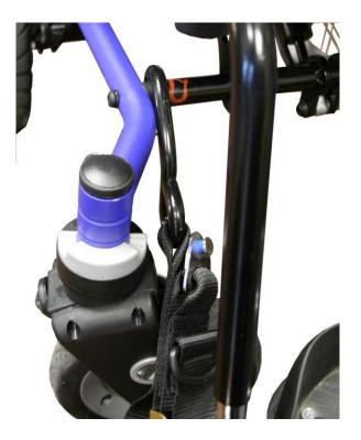
The Rear Restraints are attached to the bracket shown here
